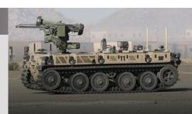
The Robotic Combat Vehicle-Light (RCV-L) experimental prototype is a small, lightweight hybrid-electric unmanned ground combat vehicle that can be transported easily by military aircraft.
